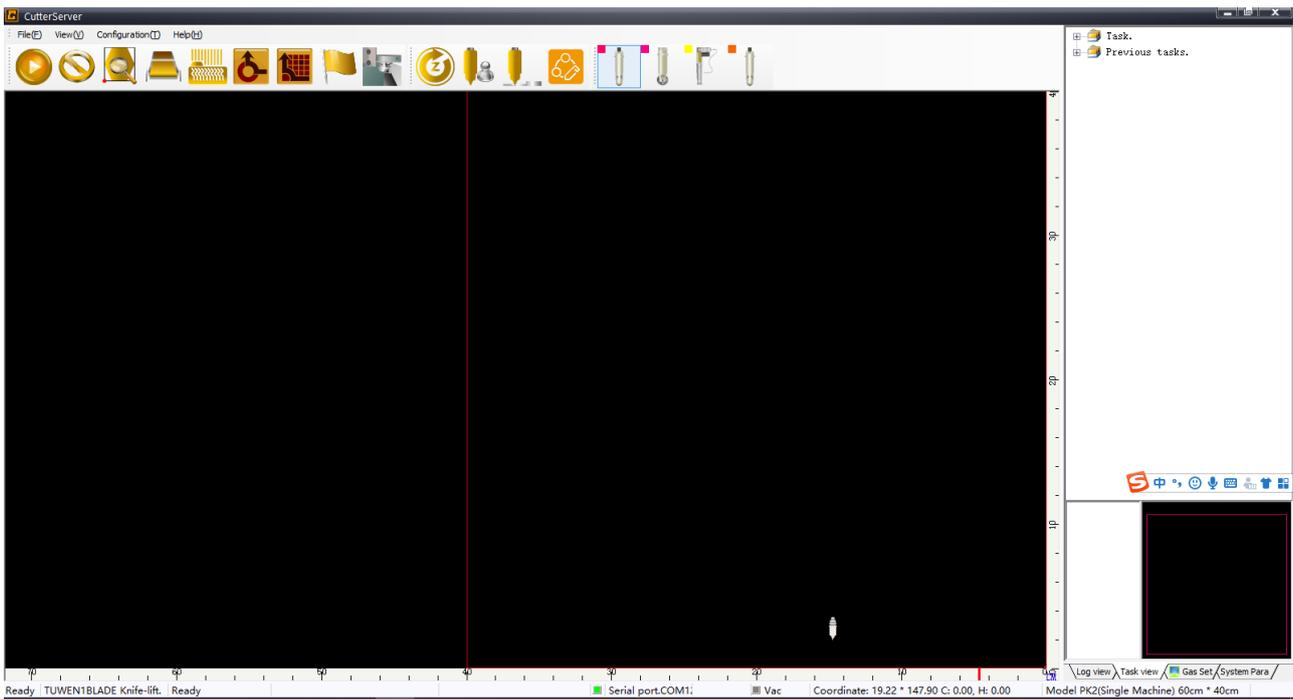
CUTTERSERVER interface in PK machines have a collecting material button icon. If cannot find it, press Ctrl+Alt+Shift+C, open function configuration window, add icon.
