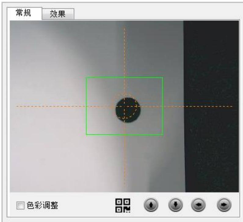
5. Click “More” in “Output settings”, open “Setting of automatic operation”. Check box “Move cutting head to the specified point before task starts”, and click Get coordinates. Then click save and exit.
